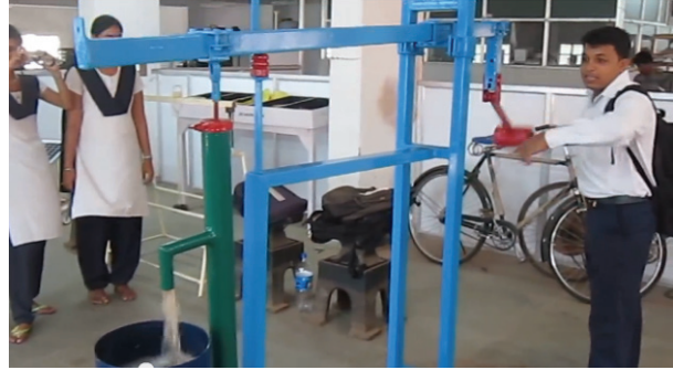
Figure 4. Replica of a hand water pump with a pendulum in India, Arun Sahoo, 2013 http://youtu.be/8n7mvpLpP5A
