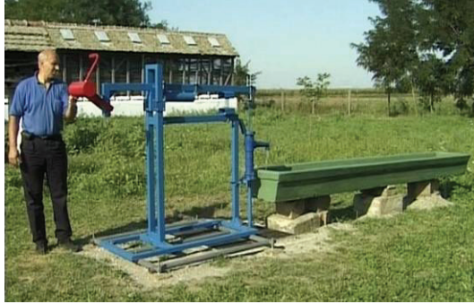
Figure 3. A hand water pump with a pendulum in a field (vicinity of Novi Sad, August 2004) http://youtu.be/hNpgl7o_1QI
