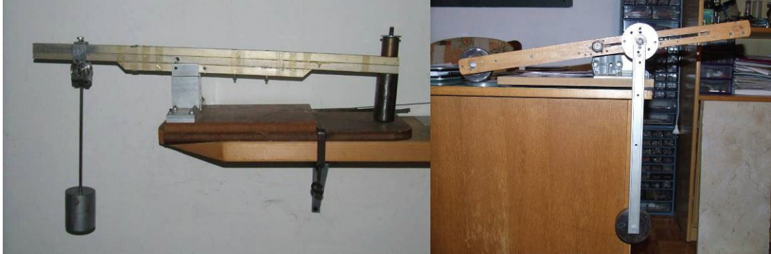
Figure 12. Mechanical hammer with a pendulum
