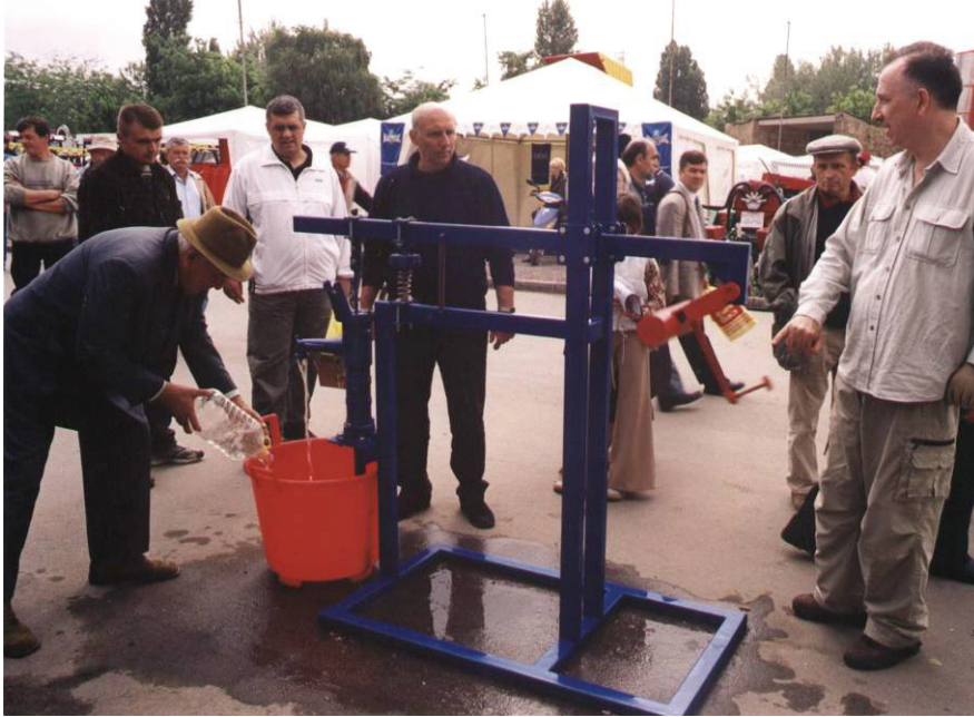
Public demonstration of mechanical advantage of pendulum-lever system Pump with a pendulum at Novi Sad fair in 2003
